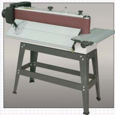
• Both working tables tilt 0-45 degree
